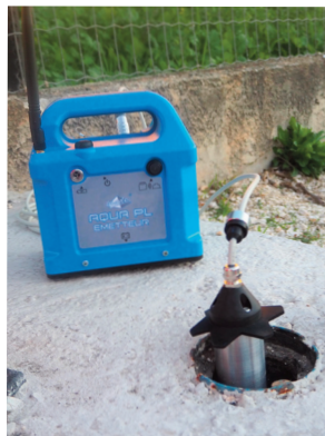
Water column injection
