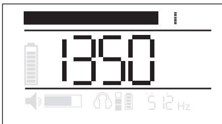
Fig. 6: Chart and numerical display of the field strength during pipe location
