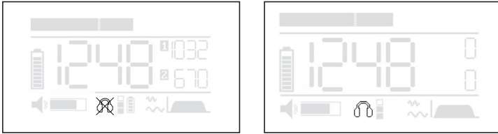
Fig. 11: Headphones symbol when the system is ready for use Left-hand figure: symbol crossed out, i.e. no measurement in progress or hearing protection threshold exceeded during a measurement Right-hand figure: symbol not crossed out, i.e. measurement ongoing
